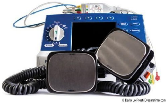
Figure 6-8 A defibrillator is used to deliver an electrical shock to the heart by means of handheld paddles or adhesive pads applied to the patient's chest.
